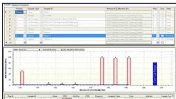
The sample run screen shown here shows a blue status bar indicating that the current sample has exceeded the defined calibration range and the intellidilution feature has been initiated.
