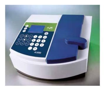
The AL800 is a modern single-beam spectrophotometer with an excellent price/performance ratio that is specifically designed for water testing.
