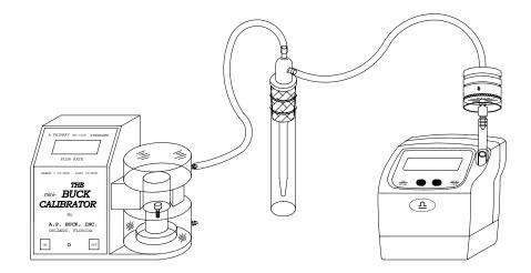
CAUTION: <u>FIRST SET THE FLOW WITHOUT SOLUTION IN</u> <u>BUBBLER.</u> The default flow rate at 2000cc/min. or previously selected flow may be too fast and draw bubbler solution into the pump. Generally, 1,000 cc/min. is the flow of choice.
